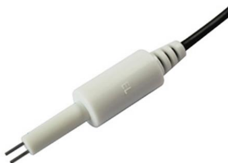
TDS probe with 2 needles
